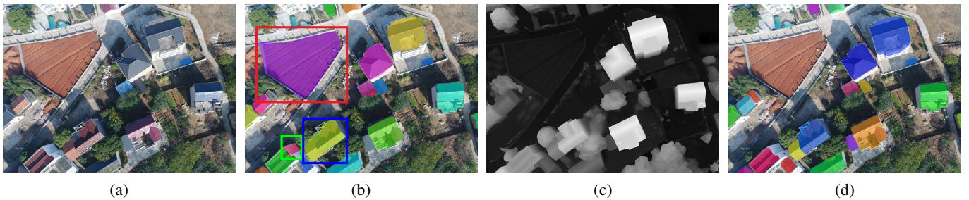
Fig. 3. Comparison of the segmentation results without and with height information. (a) An input test drone image. (b) The segmentation result using only the RGB image. The rectangles highlight three misclassified regions, i.e., a vegetable field (in red) and a wall (in green) of a building are segmented as roofs, and two roofs of attached buildings (in blue) are not separated. (c) The heightmap obtained by rendering the scene using the 3D model and the camera parameters. (d) The segmentation result using both the RGB image and the heightmap, where the vegetable field, wall, and roofs are all correctly separated.
